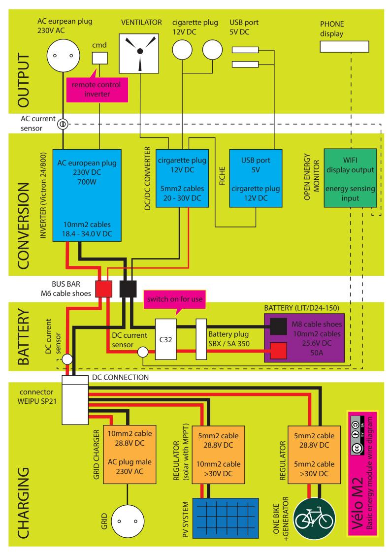
The Vélo M2 energy module can be powerd by different renewable energy sources in direct current. One of the sources is human power through pedal generation. The regulation is done by DC/DC converters that are controlling the current flow to the output. The central controller manages the power flow taking into account the state of charge of the battery and the power consumption.
